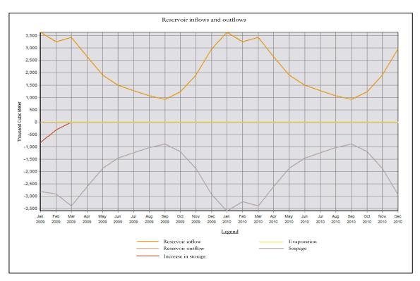
Figure 6.9 Typical reservoir in- and outflows
