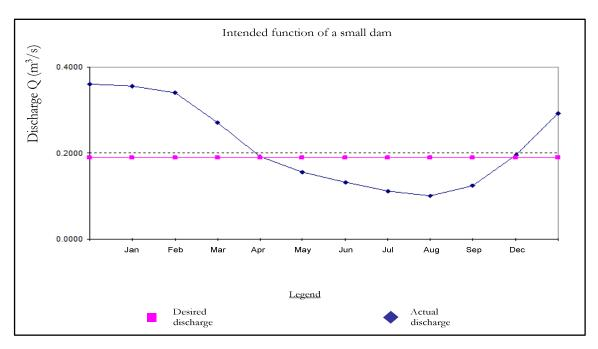
Figure 5.2 Intended regulative function of a small dam. adapted from: SEAPA (2000)
