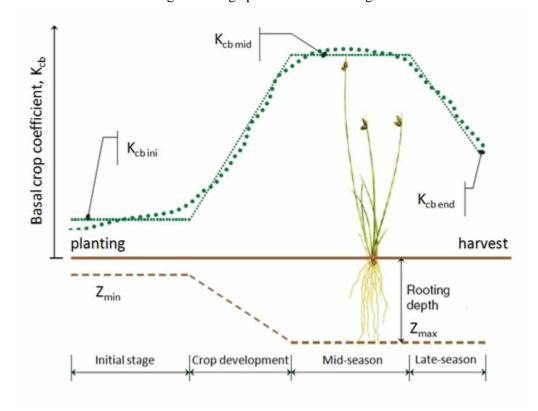
The linear K<sub>cb</sub> approximation curve is constructed by the following steps:
