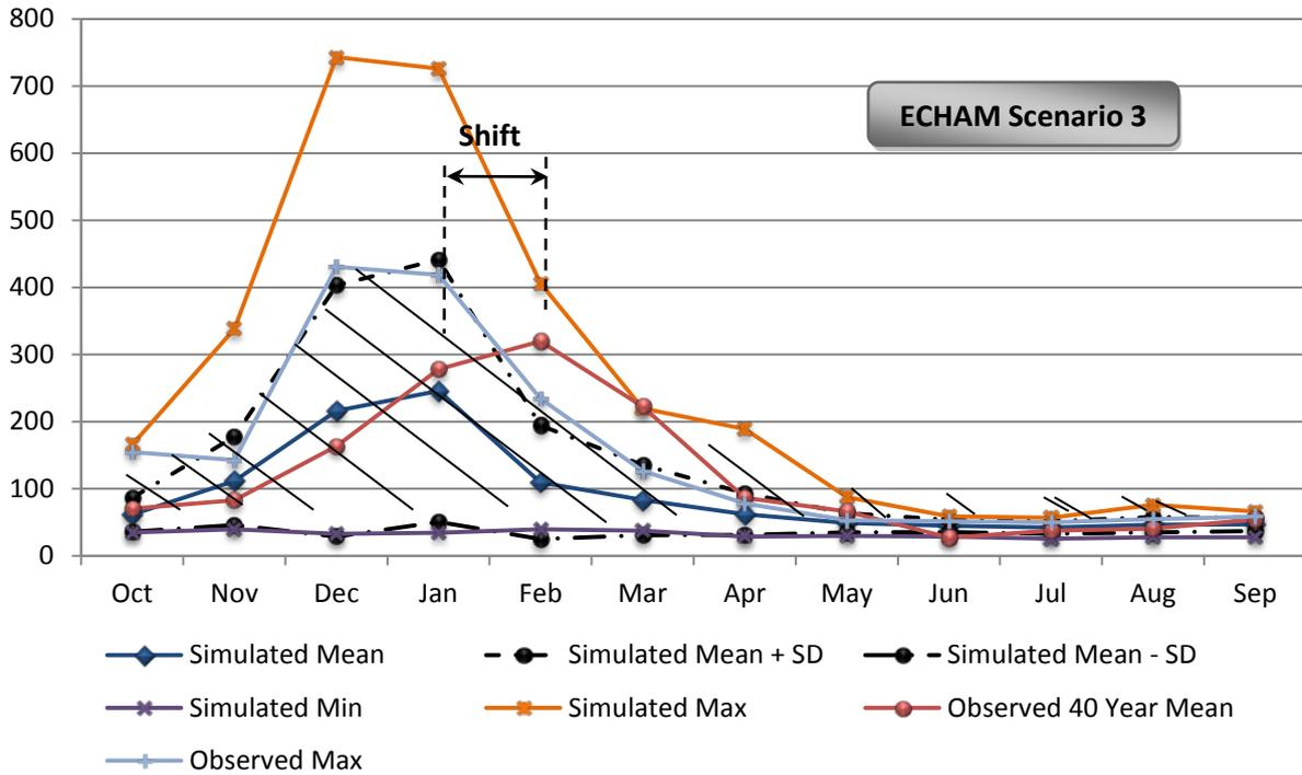
**Figure 6.45: Simulated Mean, Maximum, Minimum, One Standard Deviation under ECHAM and Historical Mean and Maximum Monthly Stream Flows**
