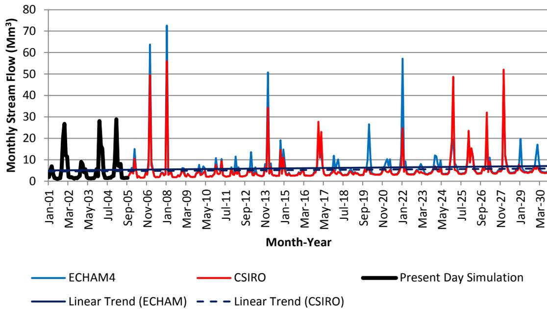
**Figure 6.35: Simulated Monthly Stream Flows for Zone 3 under Scenario 2**
