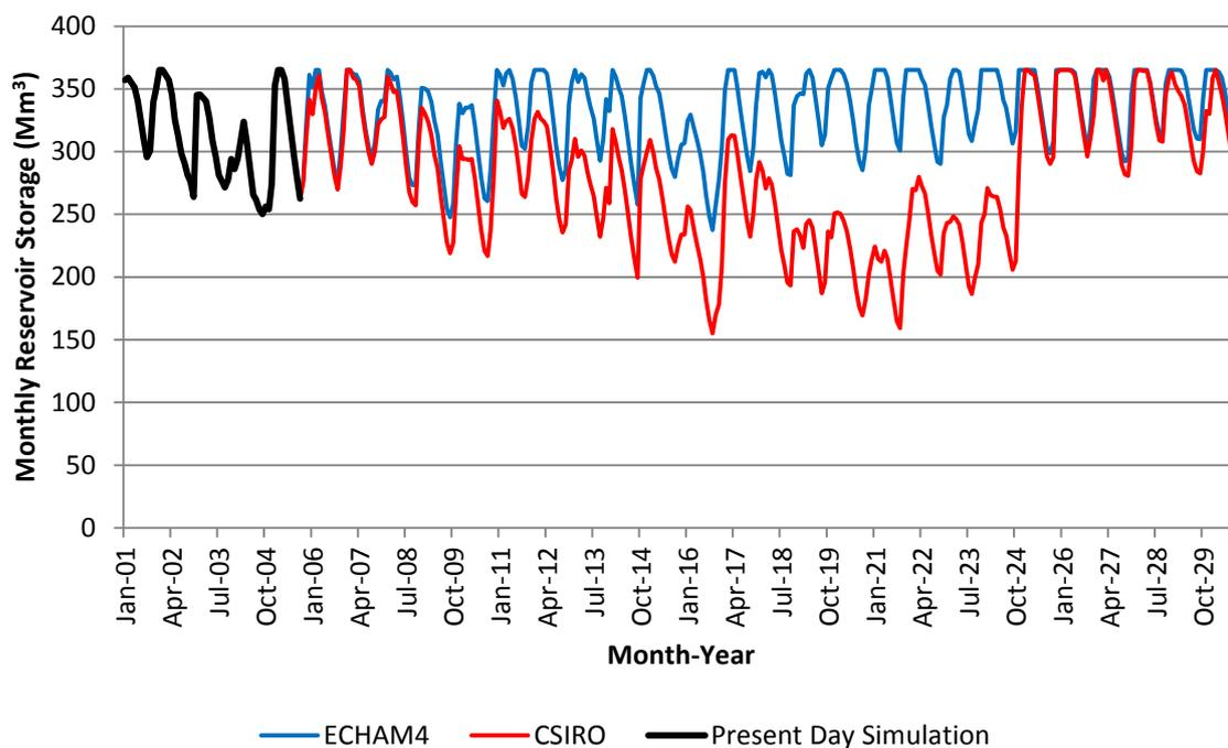
**Figure 6.50: Grootdraai Dam Simulated Reservoir Storage under Scenario 3**
