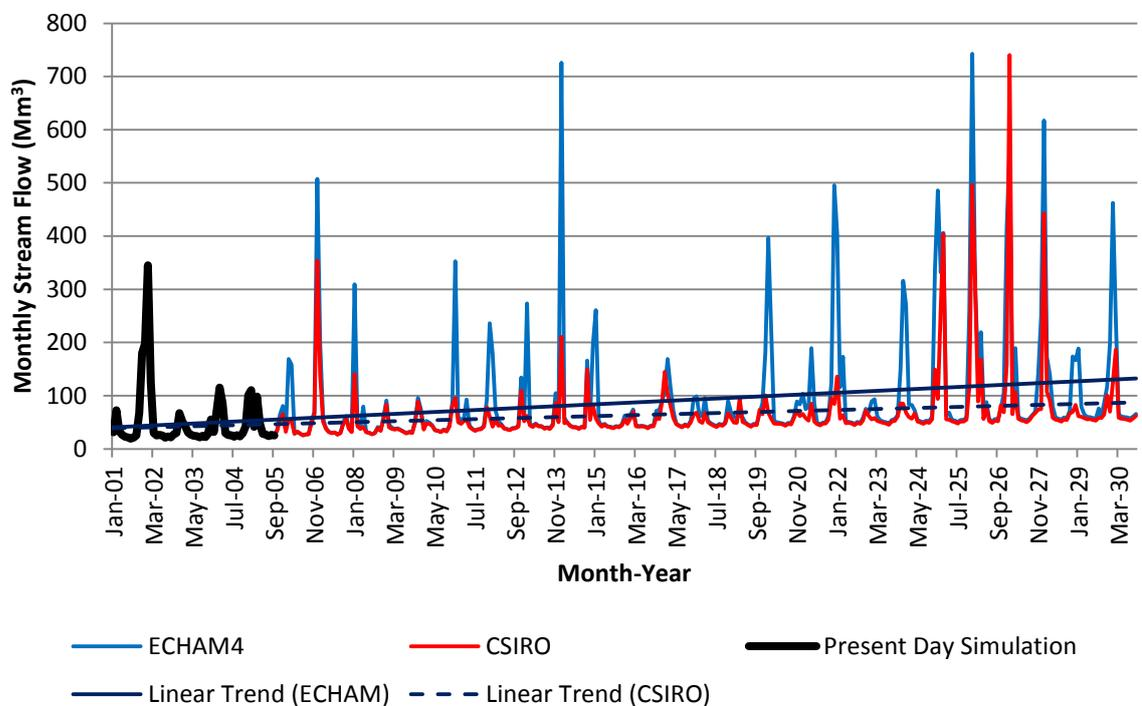
Figure 6.44: Simulated Stream Flows for Overall Basin under Scenario 3
